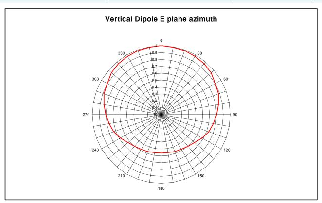
The vertical dipole antenna has a 4.7 dB front to back ratio. With an ERP of 100 Watts, the ERP at the 180 degree azimuth point would only be 33.6 Watts. So maybe the dipole is not the optimal solution.
